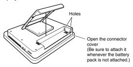
5 Insert the battery pack's catches into the player's corresponding holes. Then attach the battery pack in the direction of the arrow until a "click" is heard.
